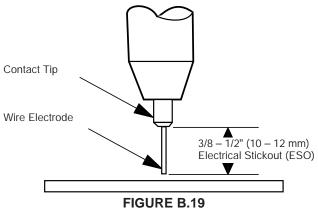
The easiest way to tell whether the ESO is the correct length is by listening to its sound. The correct ESO has a distinctive "crackling" sound, very much like eggs frying in a pan. A long ESO has a hollow, blowing or hissing sound. If the ESO is too short, you may stick the contact tip or nozzle to the weld puddle and/or fuse the wire to the contact tip.
